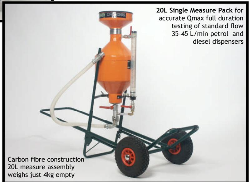
20L Single Measure Pack for accurate Qmax full duration testing of standard flow 35-45 L/min petrol and diesel dispensers
