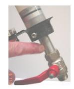
5 To bring the piston back to the required level, turn the thread using the handle of the valve.
